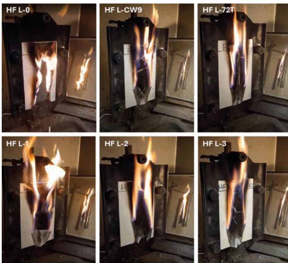
Figure 8: Vertical burning tests of different nanocomposites
