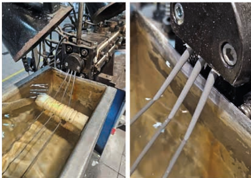
Figure 13: Extrusion before water-cutting of Dellite EFB based compound (PVC L-9).
