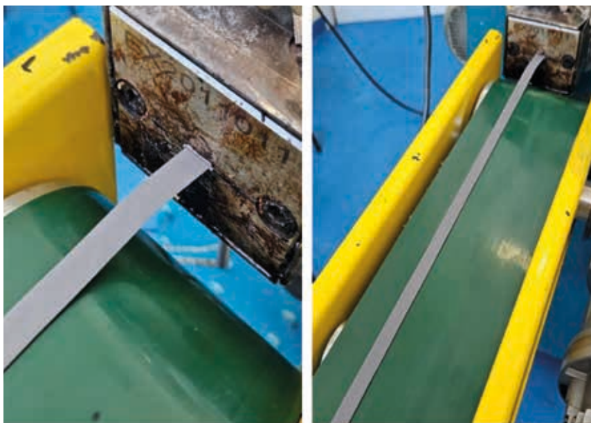
Figure 14: Flat-headed mono-screw extrusion of PVC L-9 compound.
