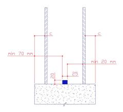
The Lavioseal HT should be held firmly in position by nails (spacing 20 - 25 cm) to ensure that the sealing strip remains in position while the concrete is poured.
