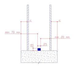
Usually the waterstop is positioned on the inside of the outermost line of reinforcing bar. This gives the required thickness of concrete to the outer surface to confine the sealing strip, avoiding any crack due to the waterstop swelling. The Lavioseal HF should be held firmly in position by nails (spacing 20 - 25 cm) to ensure that the sealing strip remains in position while the concrete is poured.
