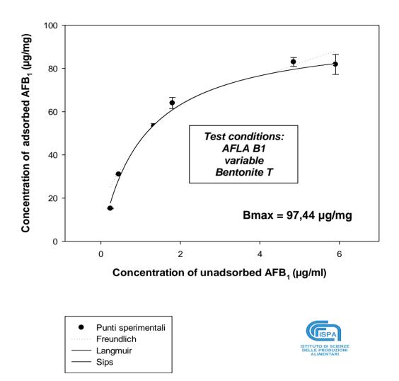
**GLOBALFEED AR** in the hydrated form has an elevated specific surface, about 800 m<sup>2</sup>/gr. This characteristic together with colloidal properties provide high adsorption behaviour and Aflatoxin control.
