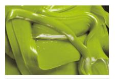
LAVIOSA ARGIMEL® organoclays are rheological additives that provide **thixotropy**: ie **thickening**, **anti-settling** and **anti-sagging properties** within solvent based systems. In particular they give:
