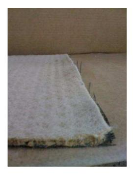
The connection between the cover and carrier geotextile is achieved by needle-punching system which enable the two geotextiles to be joined by thousands of fibres through the bentonite layer. This kind of reinforcement is especially made in order to cut down internal shear forces acting on the
