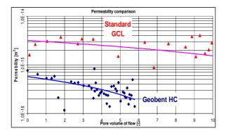
Modulo Geobent HC in presence of hydrocarbons show considerably higher performance compared to the untreated bentonite normally use in the standard GBR-C; in fact Modulo Geobent HC maintain an index flux closer to the pure Bentonite in distilled water and has a flux of one order of magnitude lower than alone bentonite in hydrocarbons hydraulic test.
