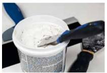
LAVIOKOLL range are powerful rheological additives developed to meet the demands of construction systems. The product advantages can be found in **improving workability, waterproofing and free-flowing characteristics**. This is due to thixotropic, antisettling and sag resistance given by processed bentonite that prevents the sedimentation of the aggregates and the bleeding of the surface.
