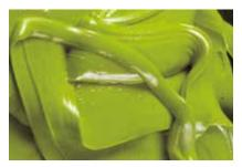
VISCOGEL® organoclays are rheological additives that provide **thixotropy**: ie **thickening**, **anti-settling** and **anti-sagging properties** within solvent based systems. In particular they give:
