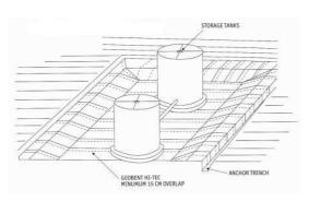
The subgrade surface shall be compacted in accordance with the project specifications. At a minimum, the subgrade should be rolled with a smooth-drum compactor of sufficient weight to remove any wheel ruts, footprints, or other abrupt grade changes. Furthermore, all protrusions extending more than 12 mm
