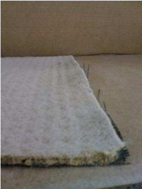
The connection between the cover and carrier geotextile is achieved by needle-punching system which enable the two geotextiles to be joined by thousands of fibres through the bentonite layer. This kind of reinforcement is especially made in order to cut down internal shear forces acting on the
