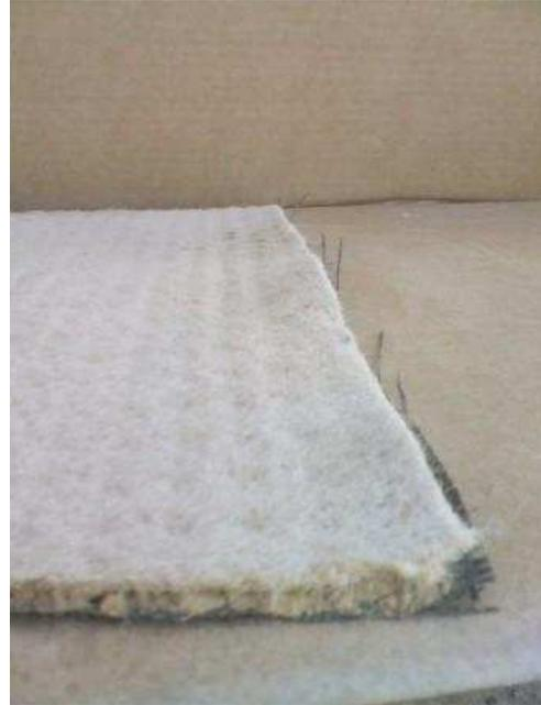
High internal shear resistance – the particular reinforcement system enable the Modulo Geobent XP to reach a strong resistance to internal friction and to be used on steep slopes providing the system with excellent stability.
